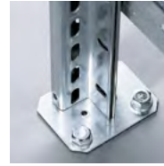
Floor attachment for shelving with a height/ depth ratio of \geq 5:1 .
